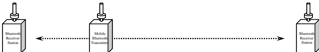
Fig. 6: Measurement setup and measured distance in meter (twice the real distance) of a moving transmitter between two receivers along a straight line; between t = 60 - 110 seconds: moving forward from receiver 1 to 2; between t = 250 - 300 seconds: moving backwards from receiver 2 to 1
