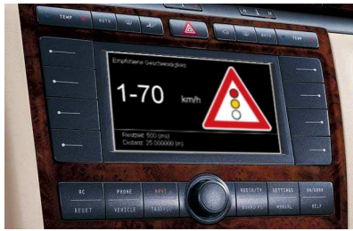
Figure 4: Information about traffic signal states and speed recommendation in the car
